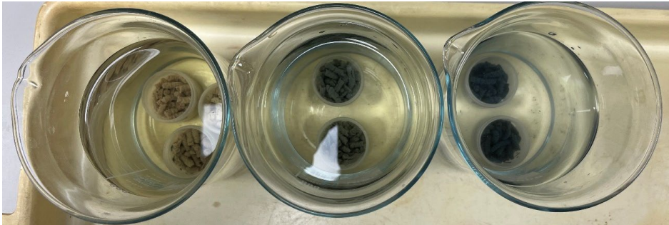
Figure 3. Study of 137 Cs sorption by feed with different hexacyanoferrate contents from an aqueous solution
